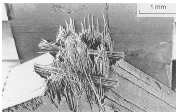
Figure 5 SEM micrographs of the two fracture surfaces, showing extensive fibre pull-out, and 90° ply failure away from the notch root.
